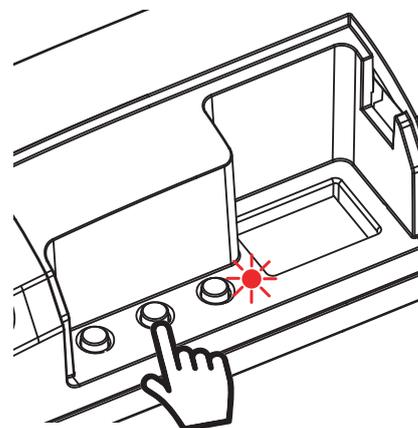
**ACTION:** Short press of button 2    **LED:** The led Flash quicly and turns off
