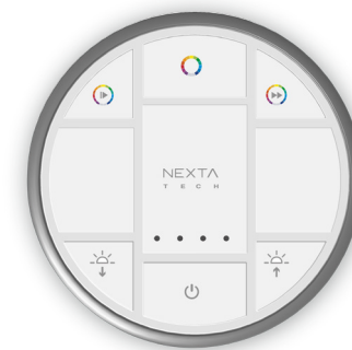
HB80-1C Radio control, rolling code 433.92 MHz, 1 channel, On-Off function, dimmer up/down, colour control RGB/RGBW and CCT, dynamic cycle control. CR2450 battery.
