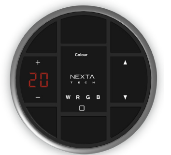
HB80-30RGBW Radio control, rolling code 433.92 MHz, 30 channels, On-Off, dimmer up/down, colour control RGB/RGBW and CCT, dynamic cycle control, open-close-stop (motor). CR2450 battery.
