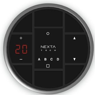
HB80-30D Radio control, rolling code 433.92MHz, 30 channels and 4 groups, On-Off , dimmer up/down, open-close-stop (motor). CR2450 battery.
