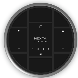
HB80-4L Radio control, rolling code 433.92MHz, 4channels + All, On-Off, dimmer up/down, open-close-stop(motor). CR2450 battery.
